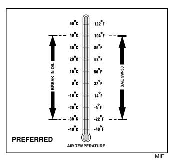
If the above recommended John Deere oils are not available, use a break-in engine oil meeting the following specification during the first 5 hours (maximum) of operation:
