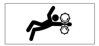
Tie long hair behind your head. Do not wear a necktie, scarf, loose clothing, or necklace when you work near machine tools or moving parts. If these items were to get caught, severe injury could result.
