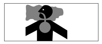
Engine exhaust fumes can cause sickness or death. If it is necessary to run an engine in an enclosed area, remove the exhaust fumes from the area with an exhaust pipe extension.
