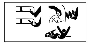
Keep hands and feet away while machine is running. Shut off power to service, lubricate or remove mower blades, augers or PTO shafts.
